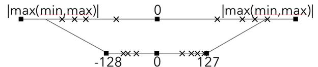
Figure 1: 8 bit quantization absmax method
