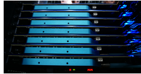
Figure 3: Seven water-cooled gaming GPUs installed on the motherboard in Figure 2.
