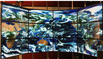
Displaying a pre-rendered ultra-hi-res visualization result of a whole earth climate simulation on 4x3 tiled displays (15360x5680 total pixels) which consisted of 12 4K displays and 4 Mac-minis. By using the newly implemented function that enables image subdivision transmission [4], we observed about 3x faster-displaying speed than SAGE2 [2]. (Data courtesy of JAMSTEC and AORI/The University of Tokyo (HPCI SPIRE3) collaboration with RIKEN AICS)
