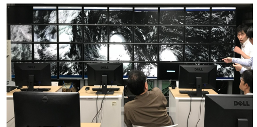
9x4 tiled displays (17280x4800 total pixels) driven by 9 Linux workstations, displaying a large-scale climate image from the weather satellite HIMAWARI-8. (Photo courtesy of Center for Environmental Remote Sensing, Chiba University and National Institute of Information and Communications Technology.)
